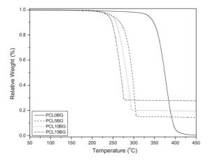
Figure 1. PCL/BG thermal degradation (TGA) curves at 5  $^{\circ}\text{C/min}.$
