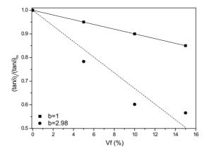
Figure 5. The  $tan \delta$  (composite)/ $tan \delta$  (matrix) versus the filler volume content (V<sub>f</sub>) in PCL/BG composites.
