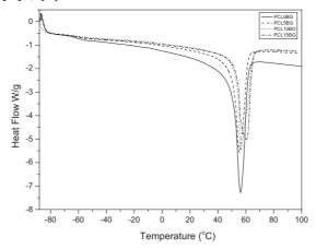
**Figure 2.**PCL/BG composites: DSC curve analysis at temperature range from −100 °C to 100 °C.
