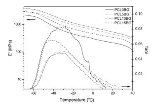
**Figure 4.** Temperature dependence of storage modulus (E') and dissipation peak ( $tan\delta$ ) for PCL/BG composite system at 1 Hz.
